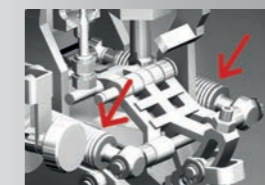
Fatigue resistant springs made of Inconel prevent malfunctions.
