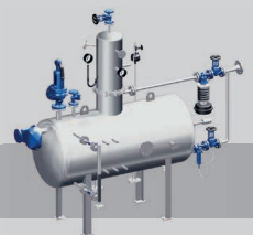
e.g. feedwater tank with deaerator dome
