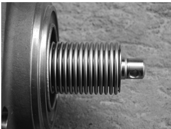
Fig. 17: Bellows of the FABA ® -Supra-C PN 40 after 200 bar water hammer
